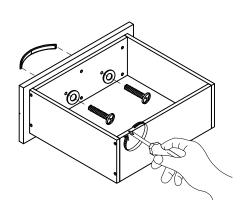
Attach handles to drawer fronts by connecting the handle to the bolt and flat washer through the pre-drilled hole and tighten with a screwdriver
